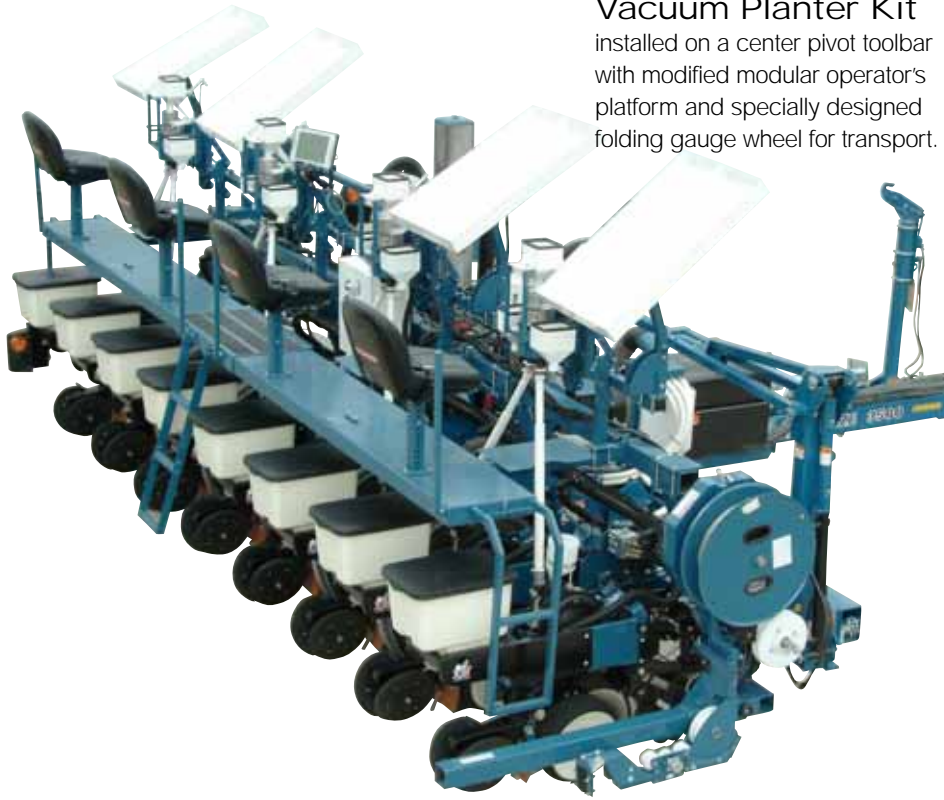
ALMACO modified gauge wheel in transport-locked position.
