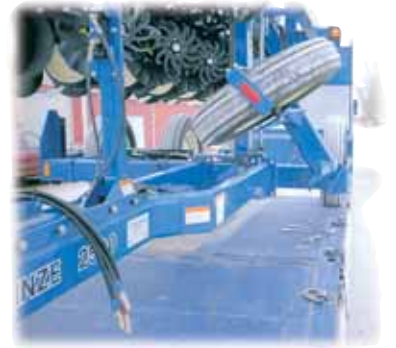
ALMACO modified gauge wheel in transport-locked position.
