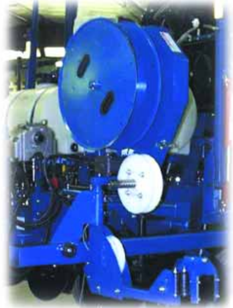
Cable Winder System mounts off planter toolbar
