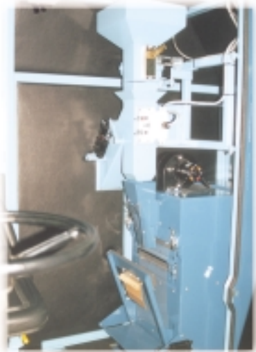
Automated Single Seed Sample Packager installed on conventional plot combine. Bags the seed from a single plot.
