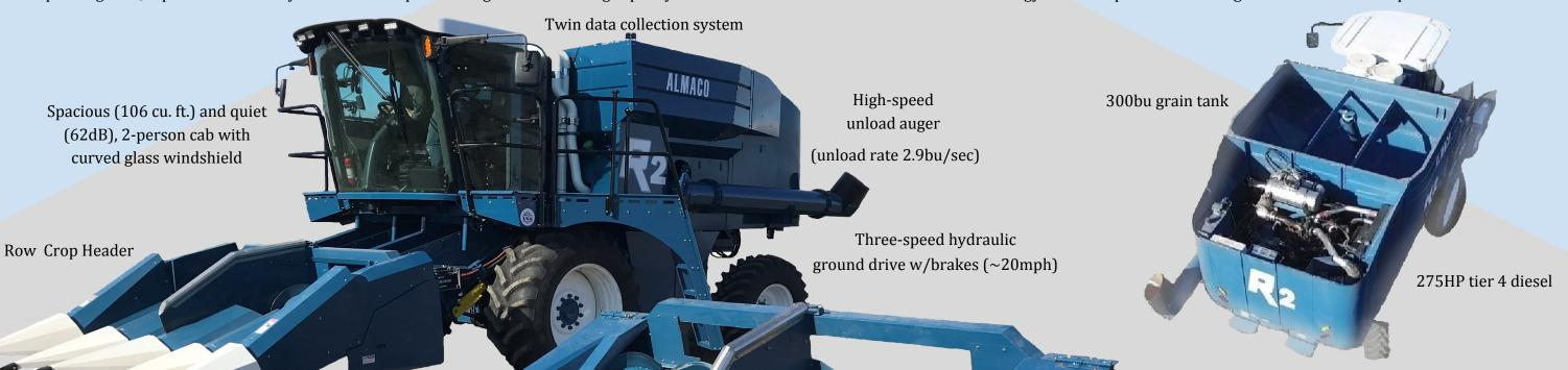
Quick-change header design for multi-crop applications. Header change in ~2-3min.
